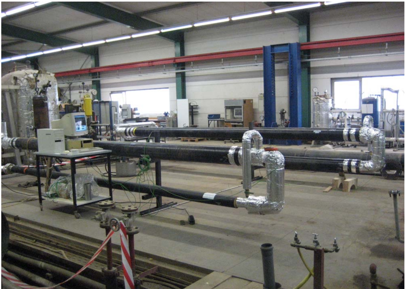
FIGURE 4 - Insulated Pipe Accelerated Heat-Ageing (CCOT) Assembly
