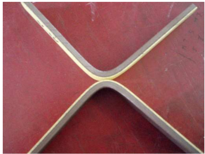
Figure 3 Samples of the new hybrid 2LPE coating after flexibility testing
