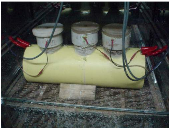
Figure 2 Cathodic disbondment resistance testing at 65°C
