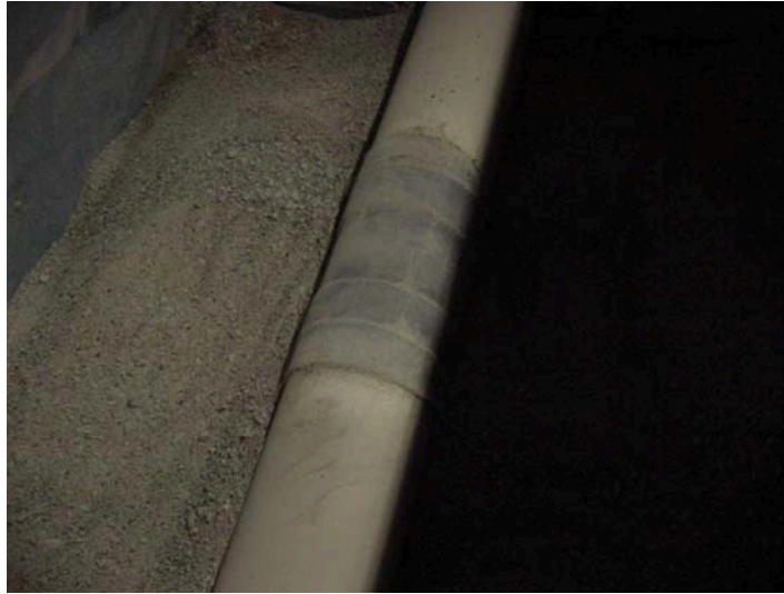
FIGURE 15 – Heat-Shrinkable Sleeve with Hybrid Adhesive Tested at 60°C for over 150 Cycles.
