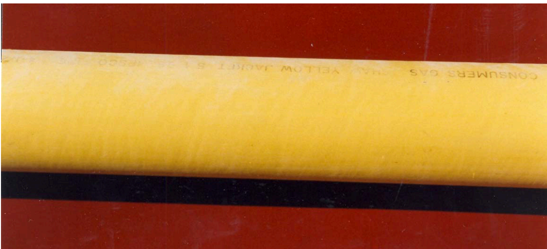
FIGURE 12 – Minor Scratches on Extruded PE Coating Surface.
