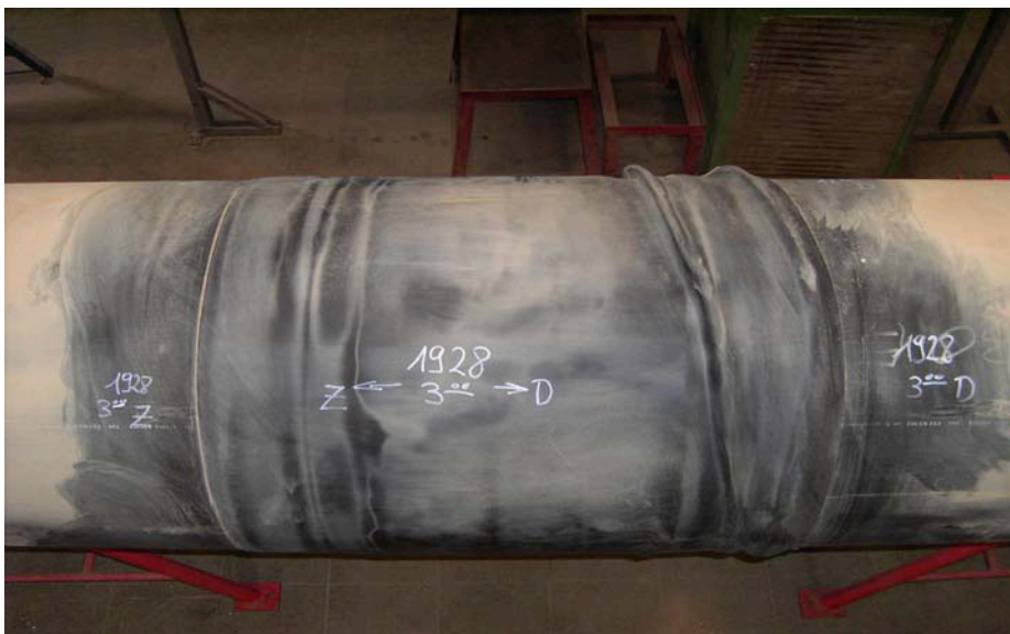
FIGURE 10 – Failure due to Low Cohesive Strength of Adhesive
