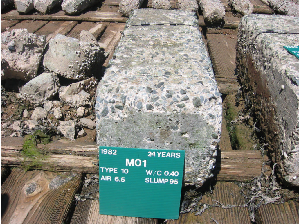
Figure 5. Phase V: : 9.3% C 3 A, 0.4 water/cement ratio (Courtesy of CANMET)
