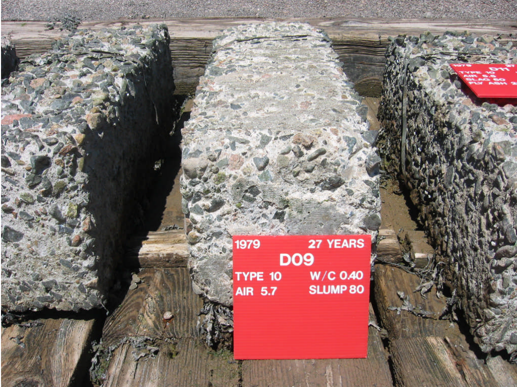
Figure 4. Phase II: 11.8% C 3 A, 0.4 water/cement ratio (Courtesy of CANMET)
