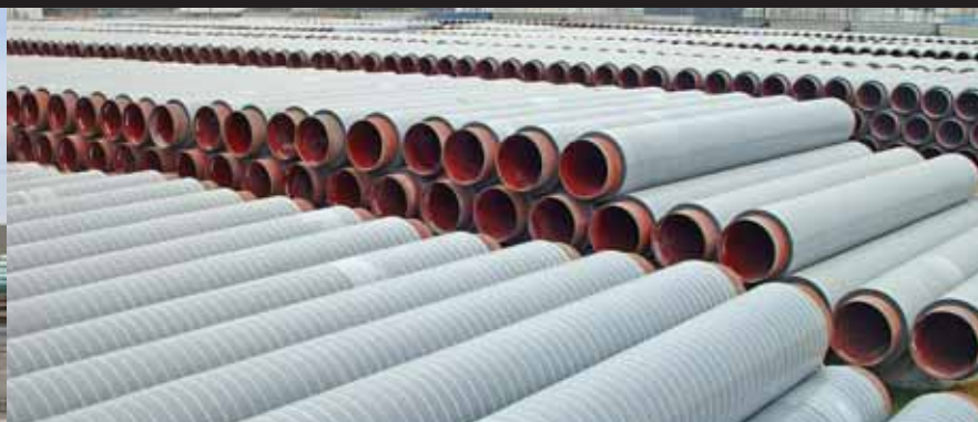
▼ Pipes Protected with Shaw Pipe's Compression Coat Technology at a Compression Coat Concrete Weight Coating Facility
