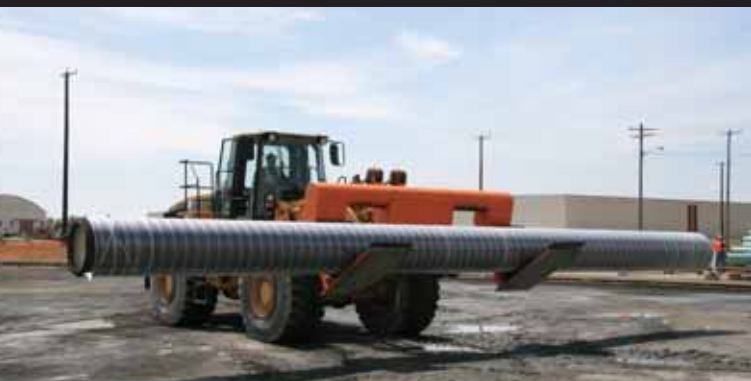
▼ Pipes Protected with Shaw Pipe's Compression Coat Technology at a Compression Coat Concrete Weight Coating Facility
