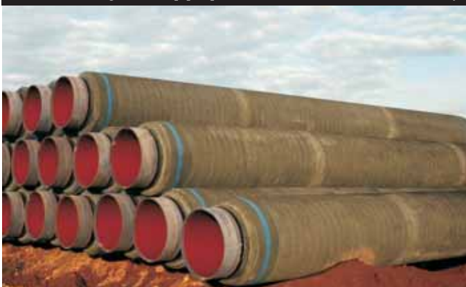
▼ Concrete weight coated pipes protected at Bredero Shaw's Leith Facility
