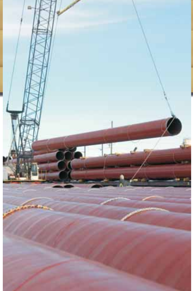
▲ FBE coated pipes protected at Shaw Pipe's Regina Facility
