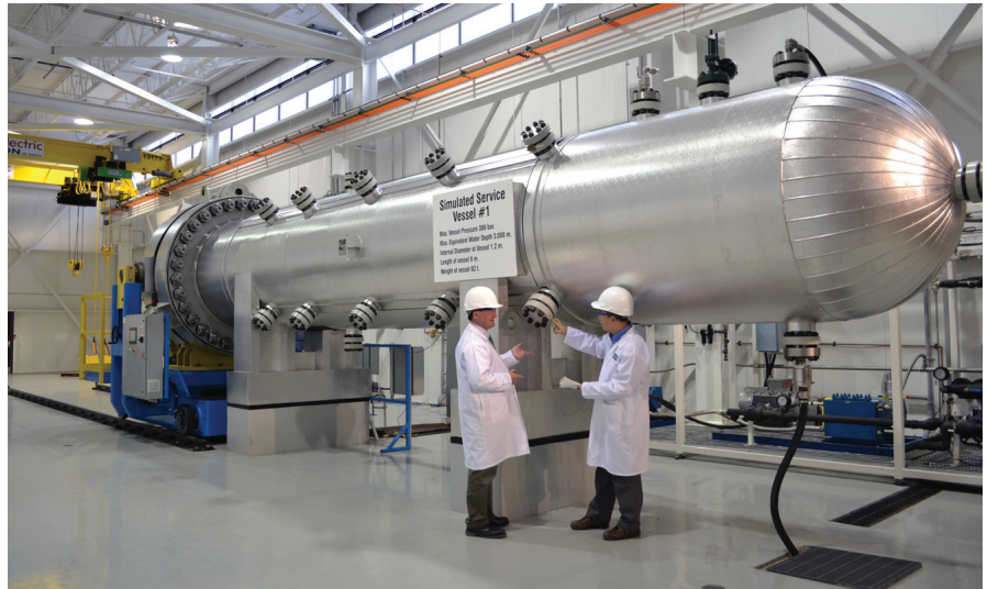
(Above) The vessel of the new subsea test facility. (Below) Door supported to meet high safety standards.
